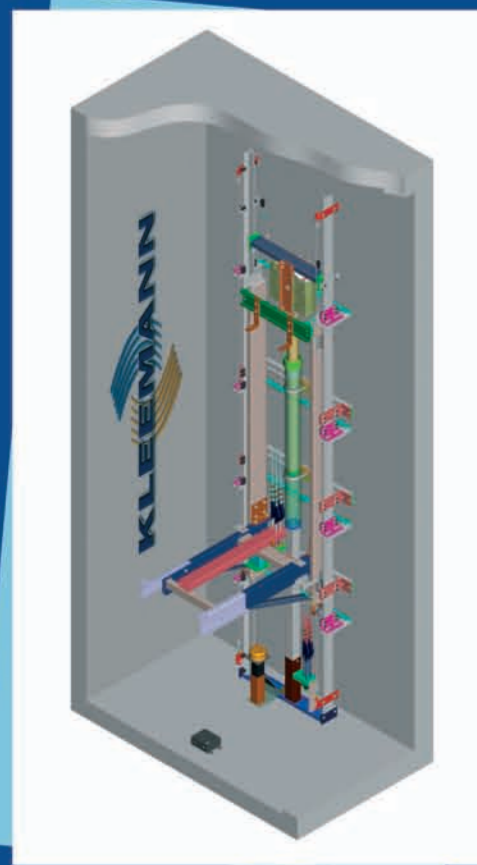
Hydraulic Earthquake resistant lift
